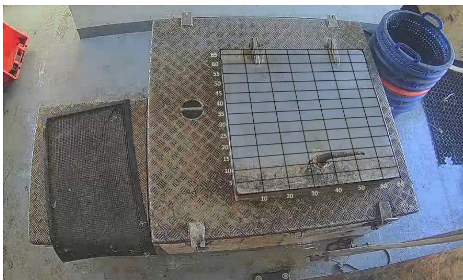
Figure. Example of a calibrated hatch onboard a commercial fishing vessel. These areas will vary from vessel to vessel, depending on available surfaces and the species being measured. This image is provided as an example from a non-tuna fishery. For tuna and tuna-like fisheries, the defined areas will have to be larger to accommodate larger species.
