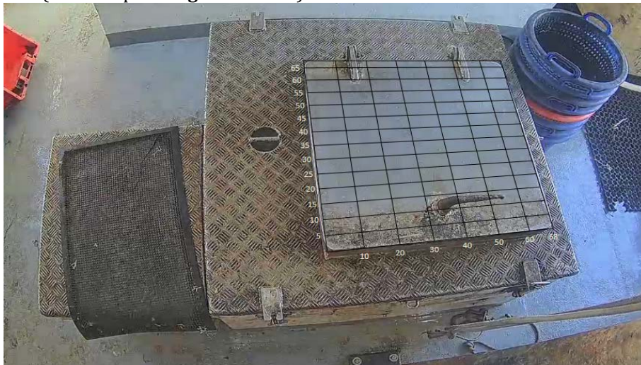
Figure 1. Example of a calibrated hatch onboard a commercial fishing vessel. These areas will vary from vessel to vessel, depending on available surfaces and the species being measured. This image is provided as an example from a non-tuna fishery. For tuna and tuna-like fisheries, the defined areas will have to be larger to accommodate larger species.
